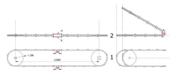
**Fig. 2** Roller chain coupled with the toothed wheels, with the portions on opposite sides replaced by ring chain portions. 1. Front view. 2. Side view. Not folded chain at the left, folded chain at the right
