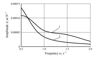
Fig. 7 Theoretical (1) and experimental (2) amplitude-frequency characteristics of oscillations of linear transverse displacement during testing of a bridge tractor as part of a harrowing control unit
