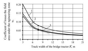
**Fig. 5** Dependence of the coefficient of losses of the field area under the engineering zone  $w_i$  on the track width *K* of the bridge tractor depending on the width of the tires of its engines:  $1 - b_{c1} = 0.586$ ;  $2 - b_{c2} = 0.429$ ;  $3 - b_{c3} = 0.394$  m
