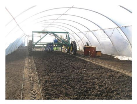
Fig. 1 Experimental studies of a bridge tractor of new construction
