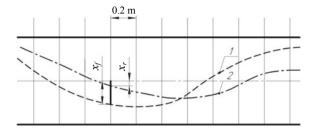
Fig. 2 Scheme for determining the transverse displacement of the bridge tractor: 1, 2-respectively, the middle of the trajectories of its front and rear wheels within the width of the technological track
