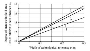
**Fig. 8** Influence of technological tolerance width *c* on the degree of field area losses under the engineering zone relative to zero tolerance depending on the width of the tires of the bridge tractor: 1 - bc1 = 0.586 m; 2 - bc2 = 0.429 m; 3 - bc3 = 0.394 m
