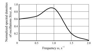
Fig. 6 Normalized spectral densities of oscillations linear transverse displacement of the bridge tractor
