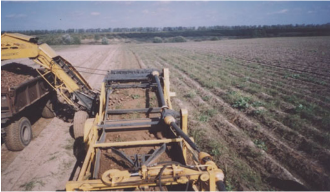
Fig. 2 Advanced design of a double-row experimental potato digger-loader (equipped with a heap leveler-distributor)
