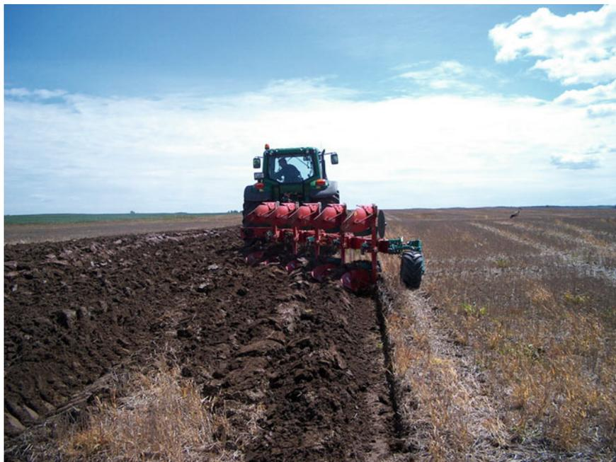
**Fig. 1** Ploughing with a reversible plough
