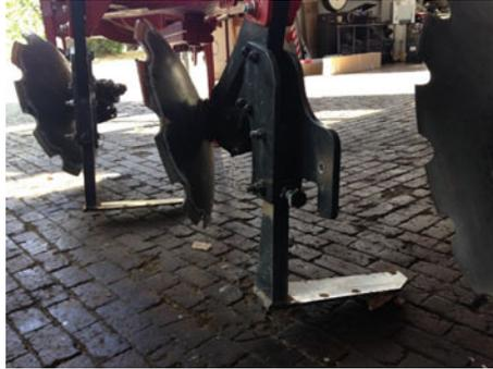
**Fig. 2** Cambered disc with knife blade for horizontal soil cutting
