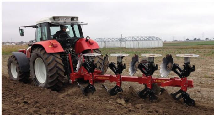
**Fig. 1** Hybrid plough (cambered disc and disc for horizontal soil cutting)
