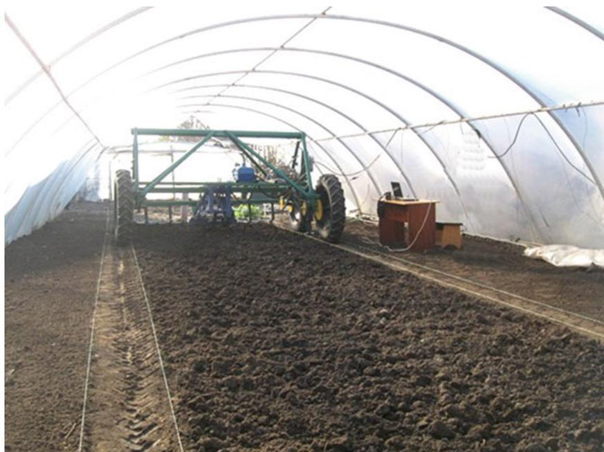
**Fig. 1** Experimental studies of a bridge tractor of new construction
