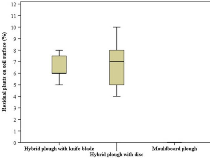
**Fig. 6** Soil coverage with residual plants in different tillage treatments. Boxplots with median. Experimental site: Raasdorf
