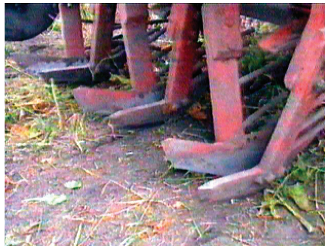
Figure 7.5. Vibrational lifting tools of experimental unit.
