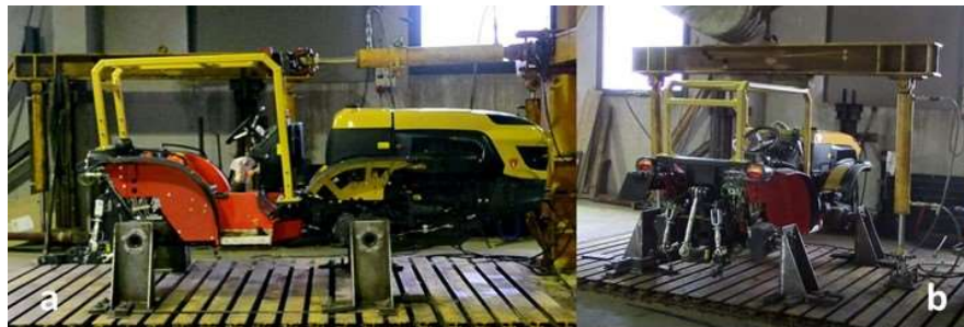
Fig. 3. The tractor ROPS at the end of the front loads: longitudinal (a) and vertical (b).
