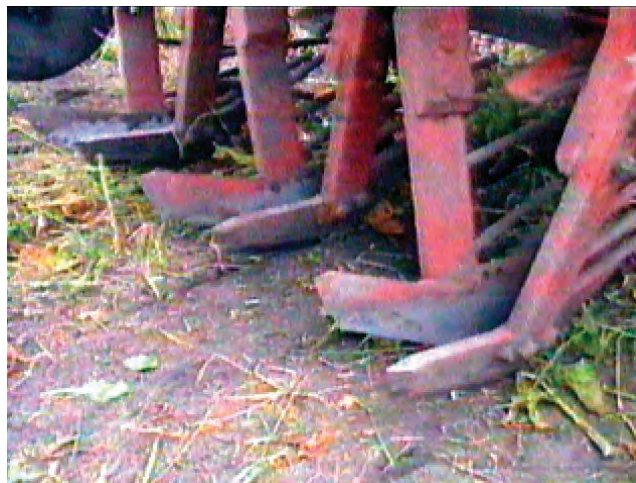
Figure 7.5. Vibrational lifting tools of experimental unit.
