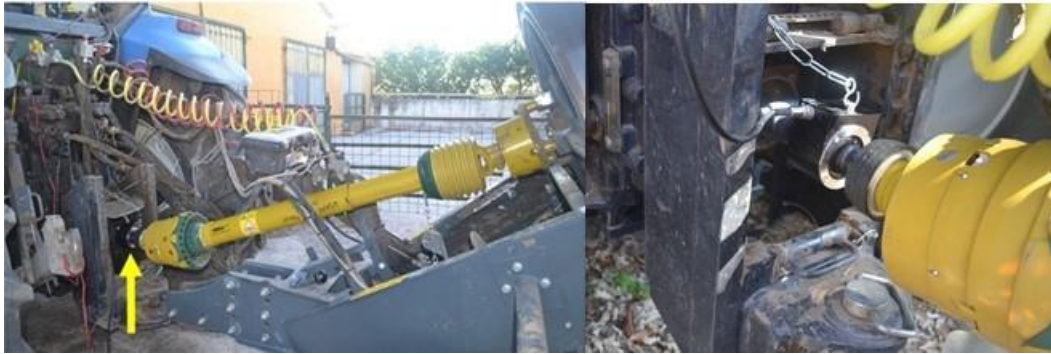
Fig. 3. Torque and speed transducer linked to the tractor PTO
