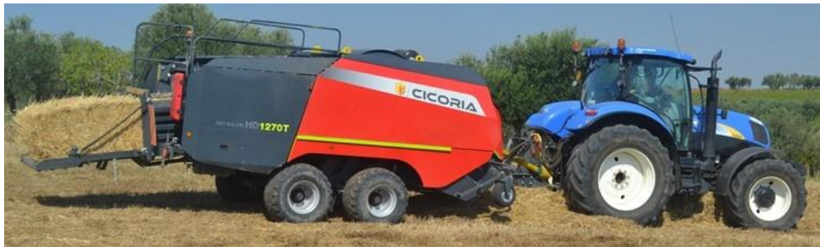
Fig 1. Big square baler Cicoria HD 1270T trailed by tractor New Holland 6090 during the tests
