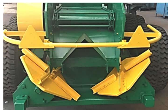
Figure 2. General appearance of prototype fertiliser spreading tools with tilted axes installed in improved-design machine for top dressing with mineral fertilisers.
