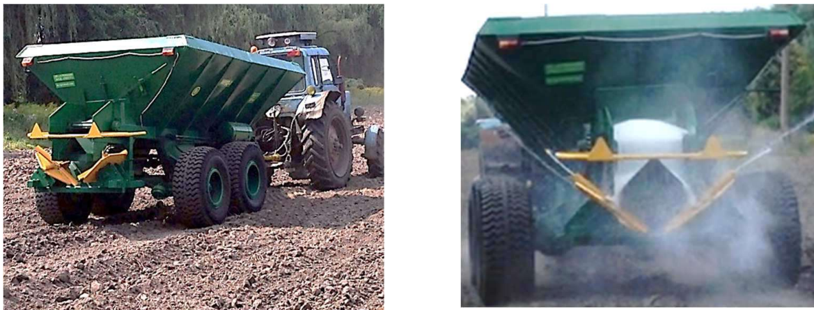
Figure 1. General appearance of improved-design machine for top dressing with mineral fertilisers, lime and gypsum equipped with two fertiliser spreading tools with tilted axes during its field testing and field experiment investigation: a – side view; b – rear view.
