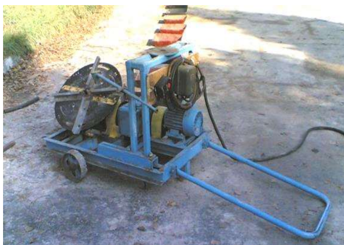
Figure 2. Experimental unit for research into process of mineral fertiliser top dressing with the use of centrifugal-type spinning-disk fertiliser spreading tools with tilted axes, with standard trays placed along the line of spreading.
