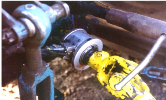
Fig. 3. Strain gauge sensor, mounted on the cardan shaft of the aggregating tractor
