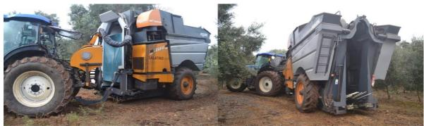
Figure 1. Towed olive harvester CV5045 built by Pellenc
