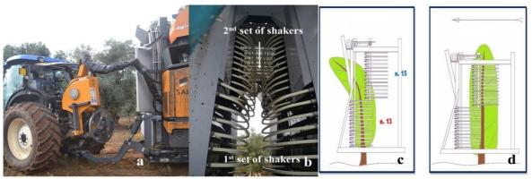
Figure 2. a. Hydraulic system to control the trim of the machine; b. Set of shakers; c. Plant into the lower shakers; d. Plant into the upper shakers.
