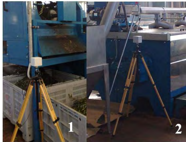
Figure 2. Measure instrumentation positioning at leaf remover out (1) and at malaxer machine in (2).
