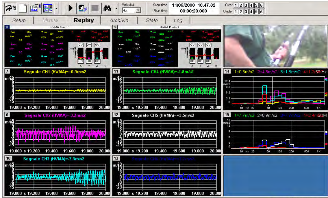
Figure 4. Signal analyses coming from the accelerometers displayed in real time
