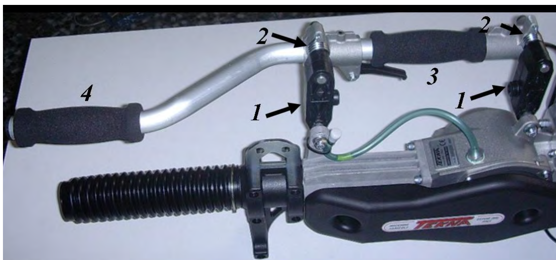
Figure 2. Vibrotek TK 5000: 1 – connecting rod, 2 – spiral spring, 3 – control hand-grip, 4 – auxiliary hand-grip
