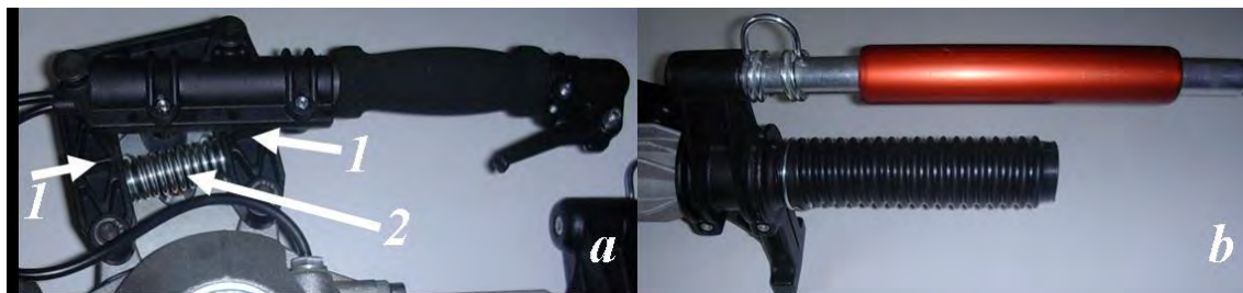
Figure 1. Vibrotek TK 650: a – control hand-grip (1 – connecting rod, 2 – spiral spring); b – auxiliary hand-grip
