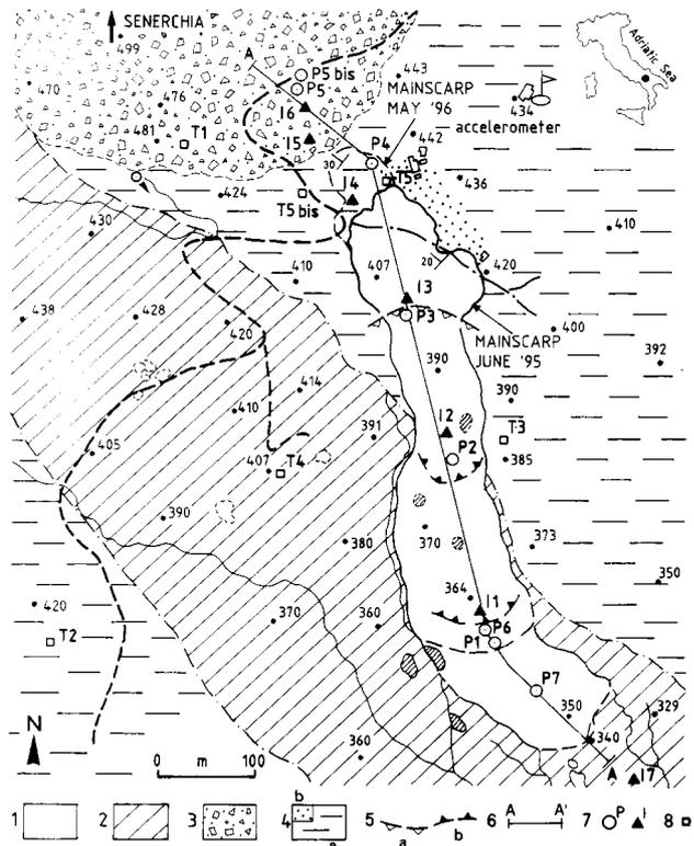
Figure 1: Geomorphological map of the slope - 1, 1993-'95 Vadoncello landslide; 2, Serra dell'Acquara earthflow; 3, debris slab; 4, a) Variegated Clay Formation, b) calcareous detritus; 5, a) 1980 crown, b) internal toes; 6, line of section in Figure 2; 7, piezometers (P) and inclinometers (I); 8, topographic control stations (after EEC Report 1996, modified).
