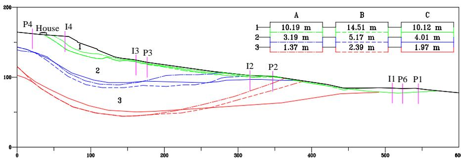
Figure 6 : Results of the numerical analysis - Areas of quasi-uniform displacement modulus (Case A: No seepage-No toe translation; B: Seepage-No toe translation; C: Seepage-Toe translation).
