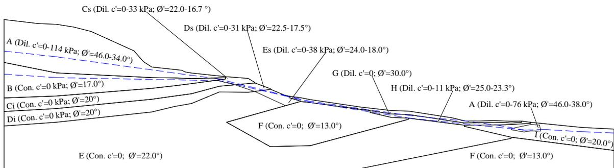
Figure 5 : Geotechnical model of Vadoncello slope; Dil.=dilative; Con.=contractant.
