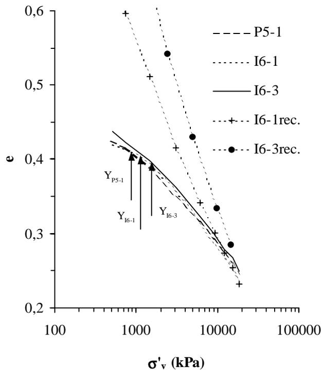
Figure 4: Natural and reconstituted samples: oedometer test results.
